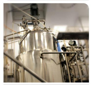
Bioreactors with volumes ranging from 50 to 5000-liter for API production
